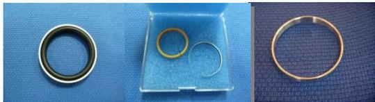
1st Displacer Seal 2nd Displacer Seal Tool, Seal Insertion
